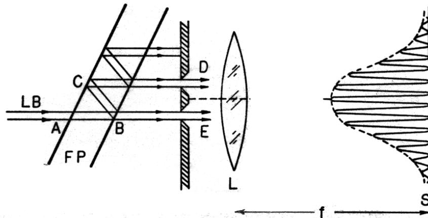
Fig. 1. Simulation of a double-slit experiment using a tilted Fabry-Perot interferometer and a laser beam. LB—laser beam; FP—Fabry-Perot; L—focussing lens;  $f$ —focal length of L; S—observation screen.
