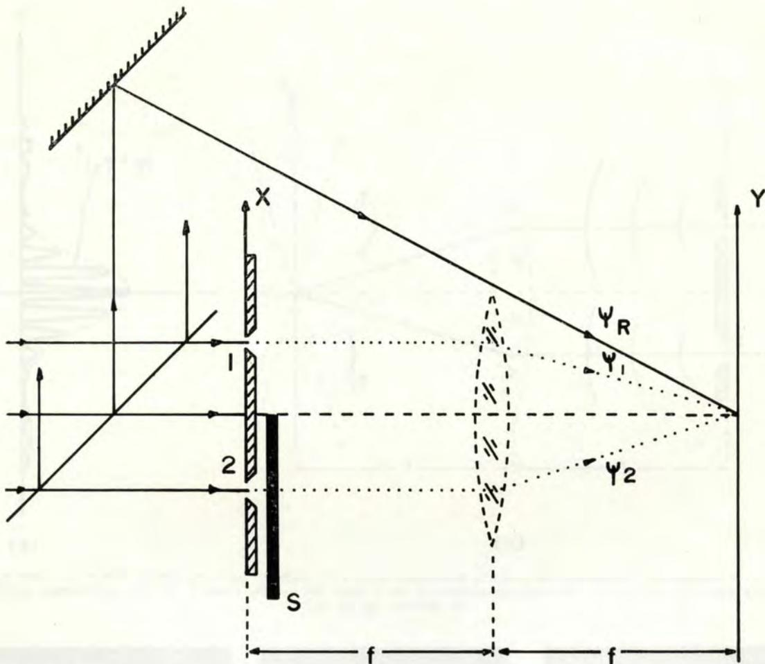
Fig. 3. Holographic experimental arrangement to record the pattern due to one slit at a time and then to reproduce the conventional double-slit pattern in complete detail.  $\psi_R$  is the holographic reference beam and  $\psi_1$  and  $\psi_2$  are single-slit waves due to slits 1 and 2.  $Y$  is the plane of the hologram.
