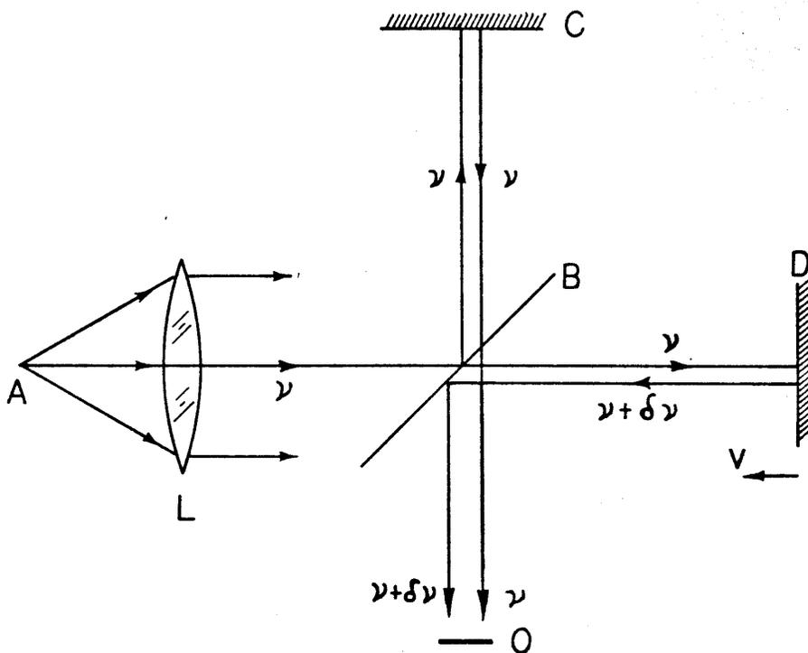
Fig. 2. Counting fringes in a Michelson interferometer with one of the mirrors moving. A—point source; L—collimating lens; B—beam-splitter; C—stationary mirror; D—moving mirror; O—observer or detector.
