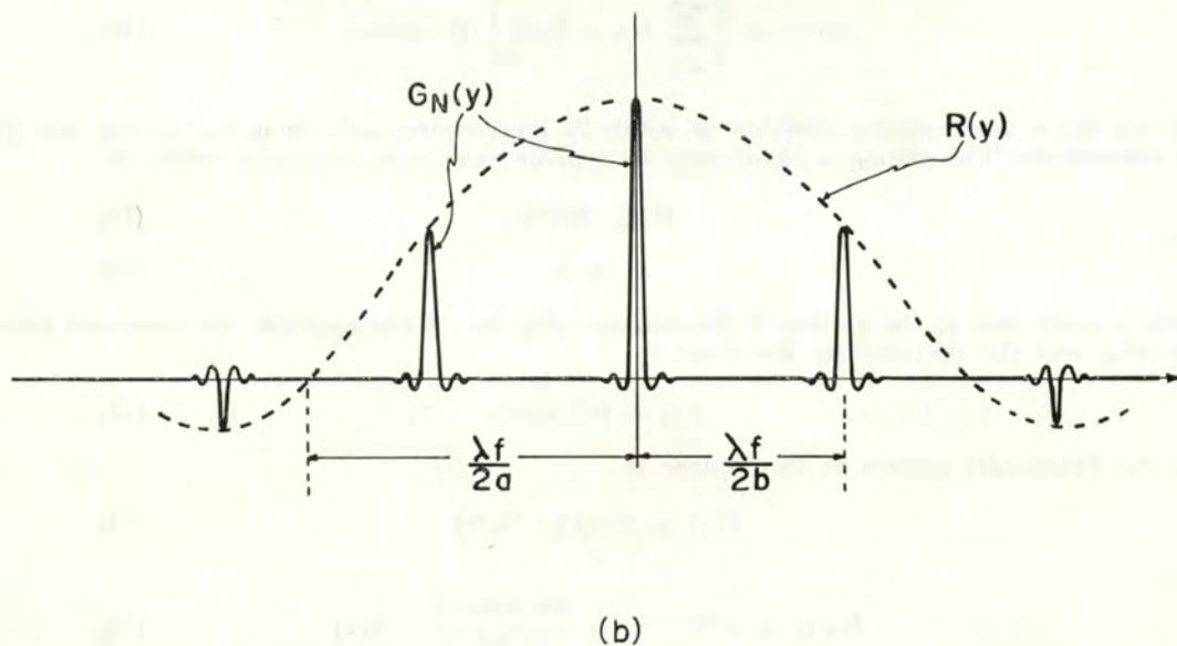
Fig. 4. Diffraction experiment with a large grating illuminated by a space limited wave-front. (a) The large grating  $g_N(x)$  is illuminated by a small wavefront  $w(x)$  at the X-plane that encompasses only a single slit. Then the observed pattern  $R(y)$  at the Y-plane is due to a single slit. (b) If the grating acts "as a whole", then the pattern should be a convolution of the single slit pattern  $R(y)$  with the N-line grating pattern  $G_N(y)$ .
