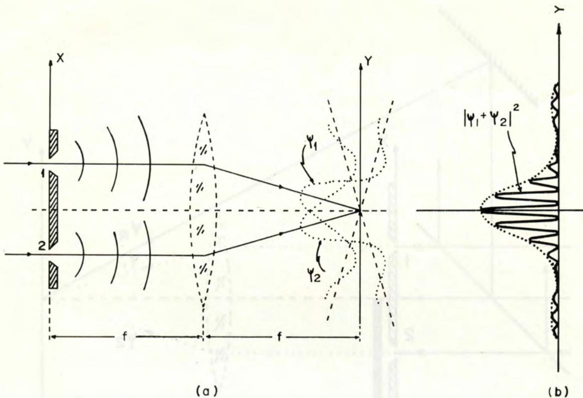
Fig. 1. A conventional arrangement to obtain a Fraunhofer double-slit pattern. (a) X-double-slit plane; Y- Fraunhofer pattern plane;  $\psi_1$  and  $\psi_2$  are two single-slit patterns at the Y-plane due to slits 1 and 2. (b) The cosinusoidal double-slit patterns,  $|\psi_1 + \psi_2|^2$ .
