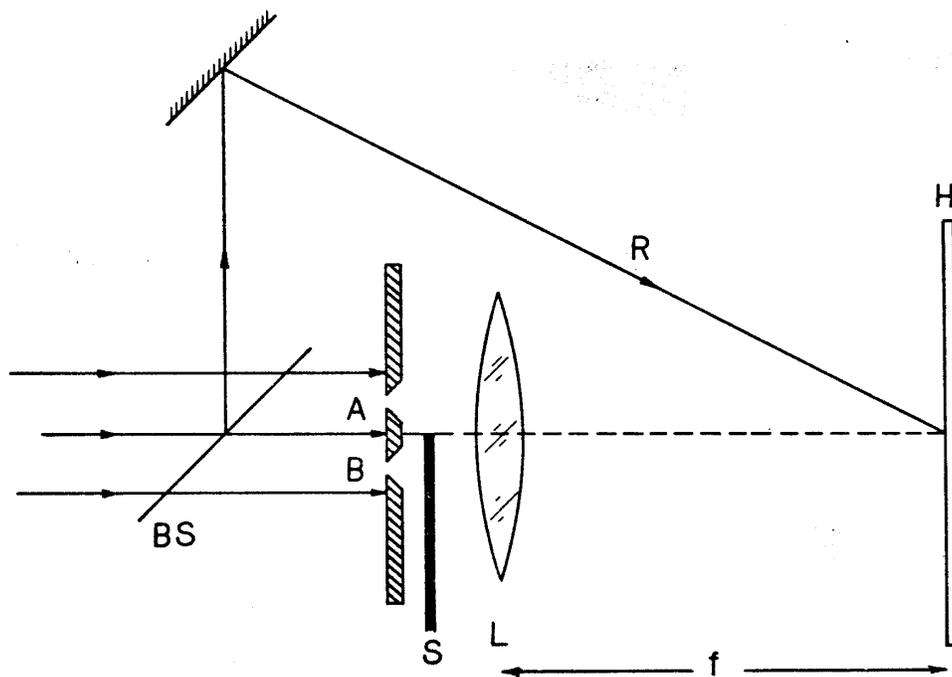
Fig. 3. Holographic recording of two individual single-slit patterns and reproduction of the double-slit pattern. BS—beam-splitter; A, B—two single slits; S—screen to cover one of the slits, A or B; L—fringe focusing lens; R—holographic reference beam; H—hologram or fringe plane.
